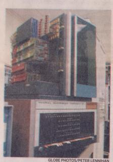
Digital's PDP-8 from 1965, recognized as the world's first commercially successful minicomputer.
